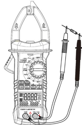
Figure 4 Schematic Diagram for Resistance Measurement at \Omega Gear
